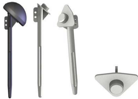
Figure 3. Different views of the SolidWorks endoprosthesis model
